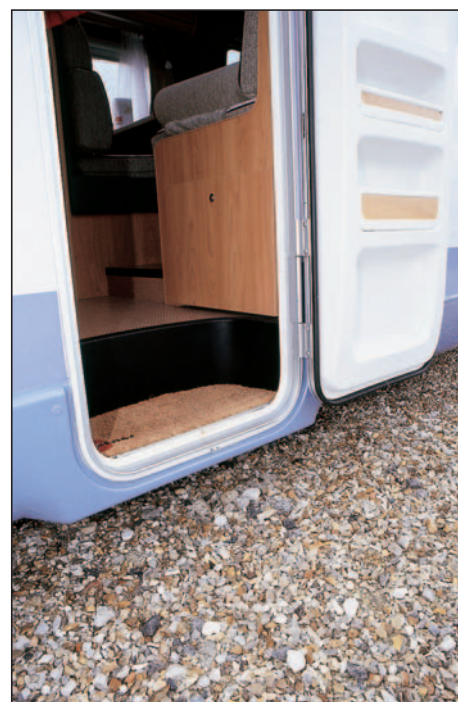
No need for a fold-out step as Renault's platform cab helps create a low caravan floor.
