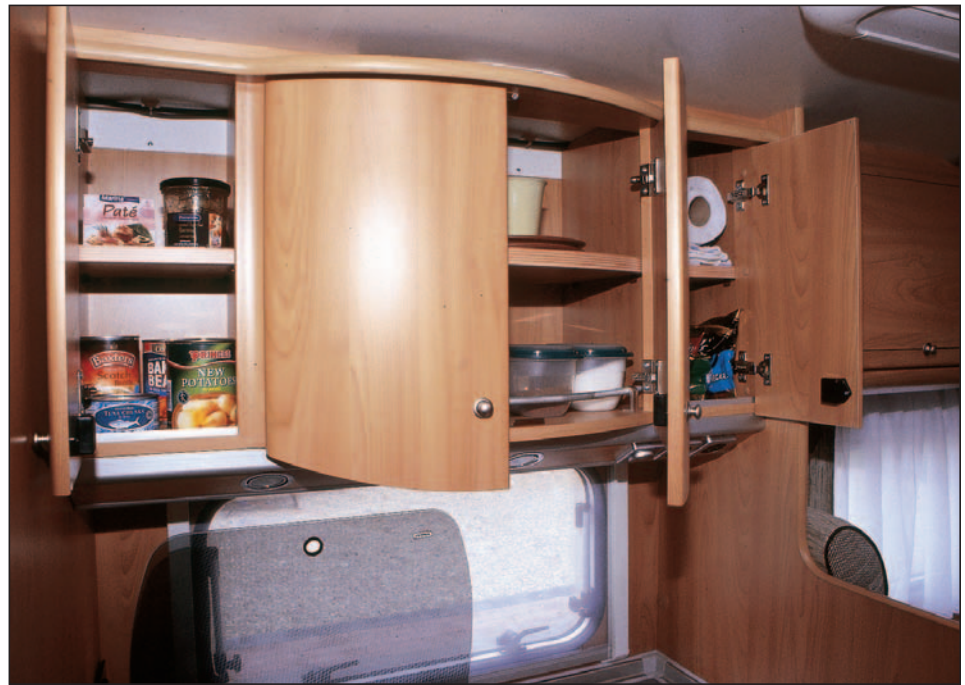
The cupboards over the kitchen have side-hinged doors – more kitchen friendly than aircraft-style lockers.
